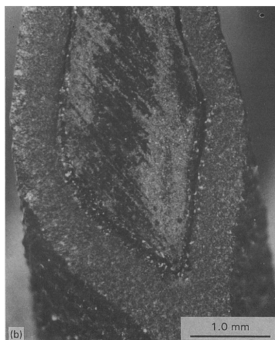
Fig. 2. Photomicrographs of the unprotected section of the new type of PbO 2 -coated titanium anode after the corrosion test in 1.53 M H 2 SO 4 at 333 K at a nominal current density of 200 A dm -2 . (a) 50 h test and (b) 1320 h test.
